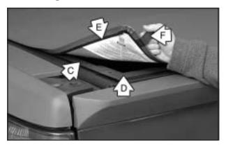
Starting at the rear corner of the driver's side of the vehicle, pull the loop (F) toward you and then pull up so the plastic lip (E) releases from the channel in the rear rail (D) and the side rail (C).
